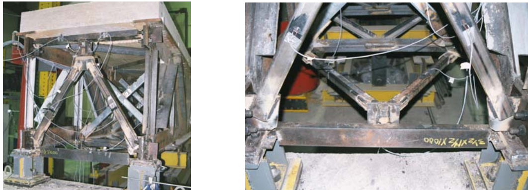
Figure 6. Retrofitted end panels of deck-truss using ductile vertical shear link
