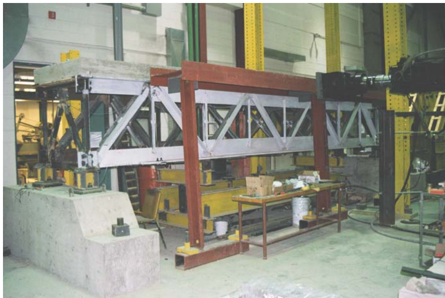
Figure 4. 27-ft long seismic retrofitted deck-truss bridge and the test set-up used for pseudo-dynamic tests at the University of Ottawa
